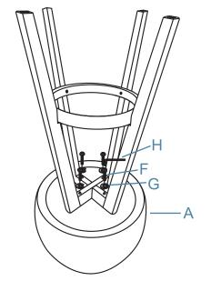
Attach assembled furniture to seat (A) as shown and secure with  $4 \times$ bolts (H) and  $4 \times$ washers (F). Tighten with an Allen Key (H).
